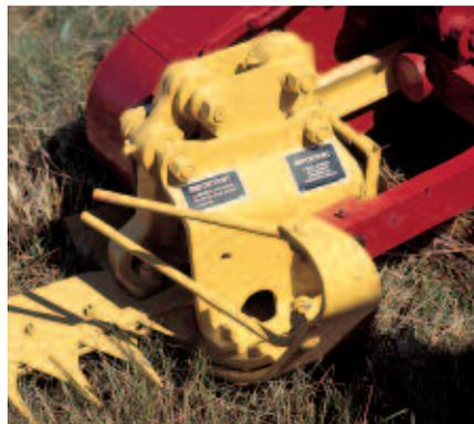
Straight-line motion of the drive head provides fast, smooth cutting combined with less wear on the knife assembly and hold-down clips.
